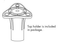
NOTE ➤ If you would like to insert a speaker stand please remove three allen screws (screw size 8mm) which are in a triangular corner. Then insert the speaker top holder carefully to avoid scraping.
