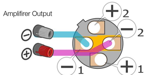
The positive misconnected to the negative which will not work.
