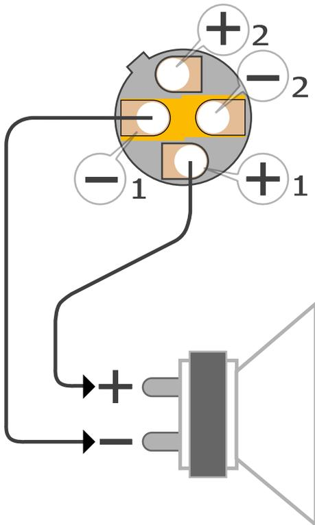
The positive and negative connect correctly to the speaker.
