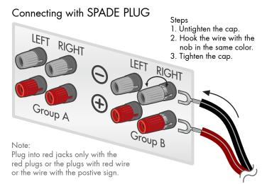
\*Note: The back panel may be placed different on actual machines; Please turn off the power and unplug the equipment before changingthe wiring configuration; Miss-connecting may damage equipments.
